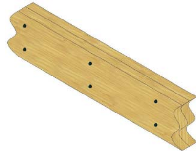
Typical connection detail of pairs of TrussLok-Z® fasteners at 24" o.c. in 2-ply LVL
