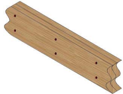
Typical connection detail of pairs of TrussLok® fasteners at 24" o.c. in 2-ply LVL
