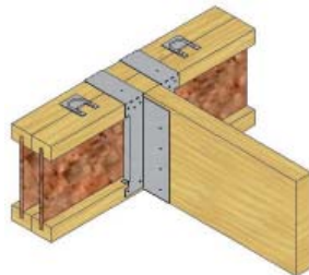
LVL/PSL/LSL or glulam to double I-Joist
